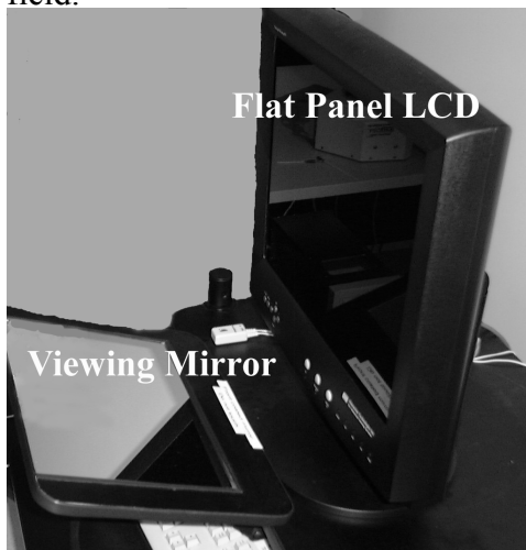
Figure 1- Demonstrates the flat screen LCD and mirror used to view the 3D rendered field.
