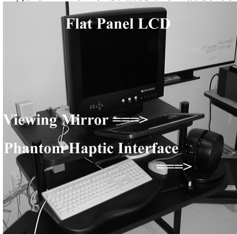
Figure 2- Demonstrates the flat screen LCD, mirror, and Phantom haptic feedback device.
